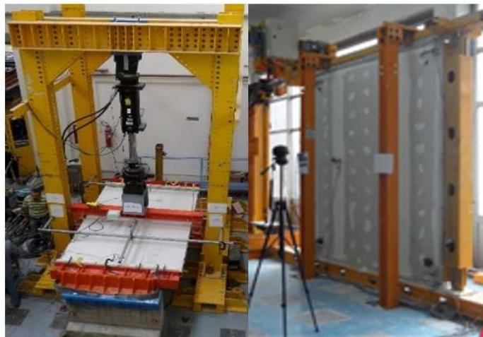
Out-of-plane partition wall tests
