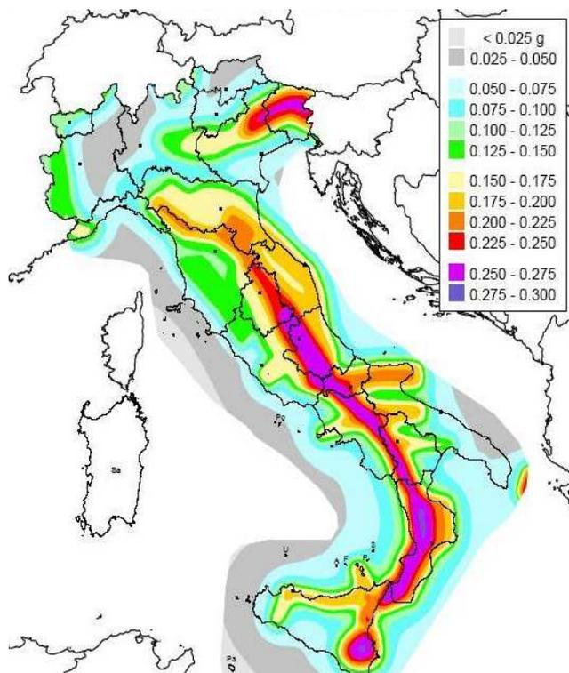
application and maintenance of storage equipment. This code introduces a new professional figure called person responsible for storage equipment safety (PRSES). In accordance with the code, PRSES must organize the warehouse and oversees structural components of steel storage racking into warehouse. In fact, new storage racking must be calculated with attention to the seismic map of Italy in accordance with last structural code called NTC [3].
