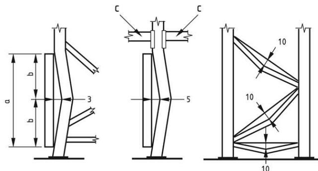
Figure 4 - damage measurements by EN 15635.
